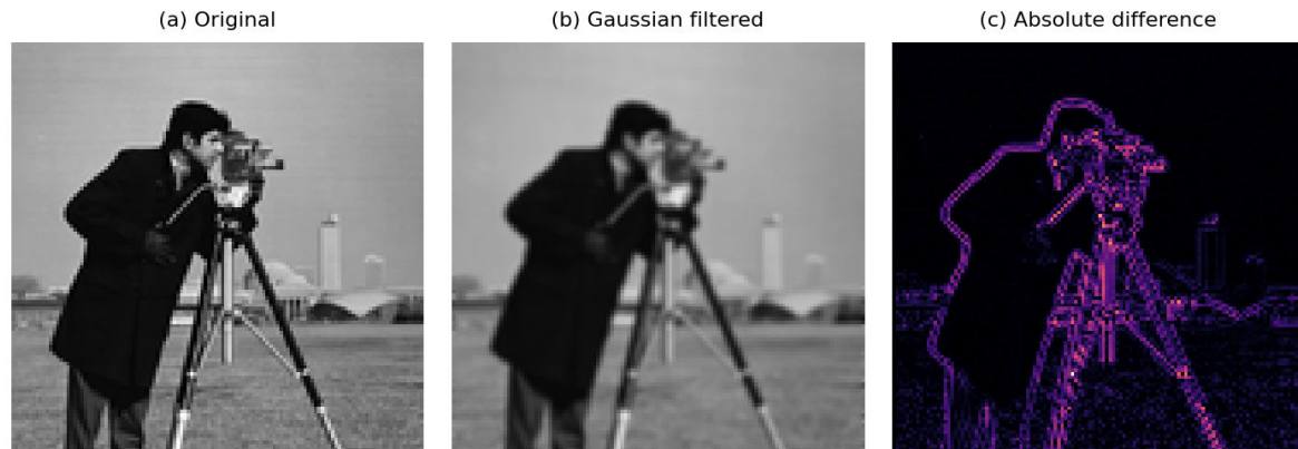
Fig. 4 (a) Original image, (b) output of the 3×3 Gaussian filter, (c) absolute difference.
